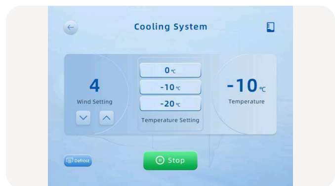
Fig. 6 — Working: wind setting, temperature set point and actual nozzle temperature.
